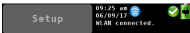
Fig.61: „WLAN connected“ appears in the upper display, alternating with the selected customer
