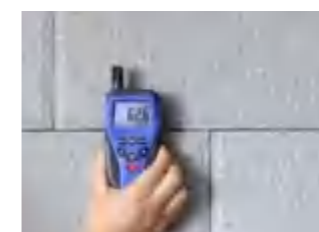
Measure moisture of wall material with non-invasive Pinless technology
